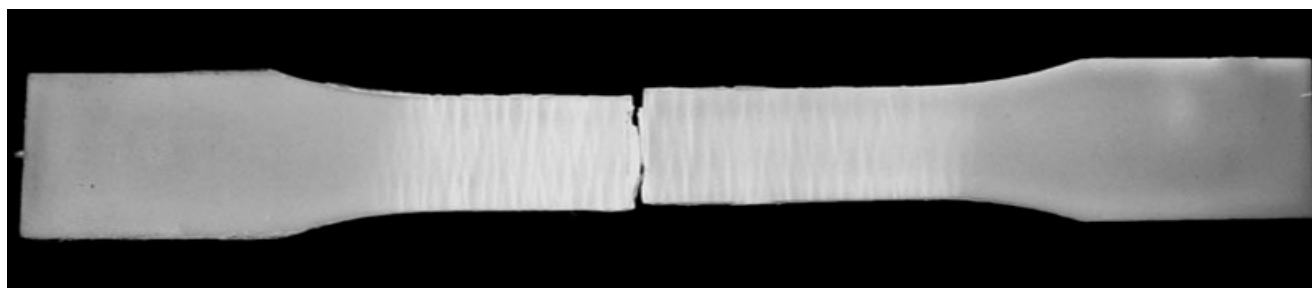
Figure 12 Macro crazes observed on the tensile fractured specimen of compatibilized PP/E20/C4 blend.
